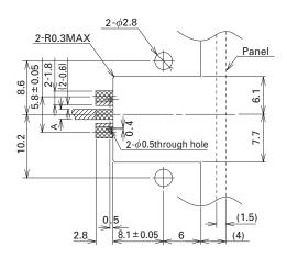
\* Set dimension A to give  $50\Omega$  characteristics. Reference example: Glass epoxy t = 1.0 ( $\varepsilon$  = 4.8) A = 1.65
